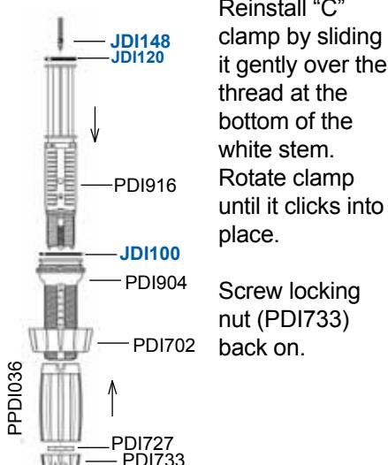
Reinstall "C" clamp by sliding it gently over the thread at the bottom of the white stem. Rotate clamp until it clicks into place.
